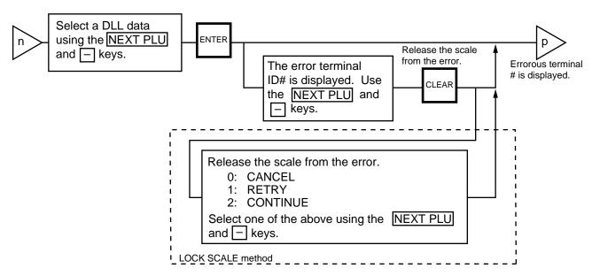
**NOTE:** DLL is performed automatically in the following two ways. It is selectable by the Initial Settings #0-6 and #0-7.
